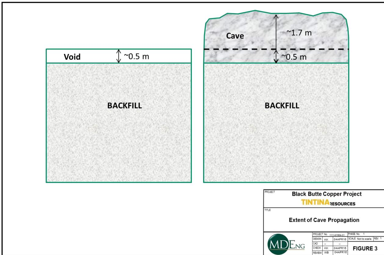
Based on the analysis presented here, it is the opinion of Mine Design Engineering Inc. that failure of the Black Butte Project LSZ crown pillar is extremely unlikely. There is no concern for long-term stability of the LSZ crown pillar, the risk of crown pillar failure is extremely low and consequence of such failure are therefore considered negligible. No rehabilitation measures will be necessary.
